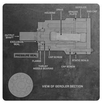
shaft seal and causes leaks. On these Char-Lynn motors, the pressure on the low-pressure return hose should not be more than 1000 PSI (6.9 Mpa) or so.
